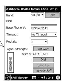
Ashtech/Thales Rover GSM Setup 900/18 🕶 Band: PIN: Base Phone #: Press 'Dial' to call on the Base station ..... 0243433141 No Timeout Timeout: and wait for GSM status 'ON LINE' Redials: Set GSM GSM STATUS: ONLINE <u>D</u>ial <u>H</u>ang Up Turn On/Off **四 ・ ■€ 10:42** 🛠 ₿ FAST Survey
